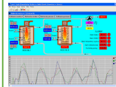
Visualization programs enabling to build distributed control and measuring systems like: RISHABH-CONTROLS, RISHABH-PROCES, RISHABH-3000.
