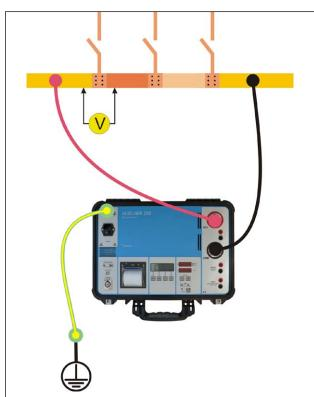
Using an external voltmeter, measure the voltage drop (voltage) across each contact element within every section of the bus-bar being tested.
