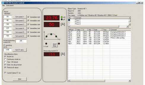
The Windows program makes it easy to manage/save all test results in a simple way. All information, meta-data of the test object e.g. a circuit breaker and the test results are stored together and they can easily be transferred to Microsoft® Excel for further analysis.
