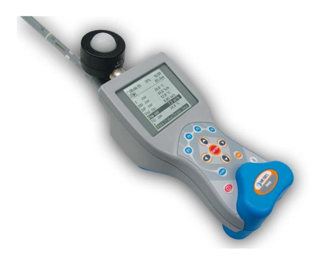
Measurement functions for air temperature, air velocity, relative humidity, illuminance and luminance are all found within one device.
