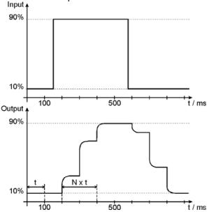
Picture 3: Output transfer characteristic
