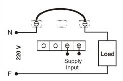
Note: Device will be damaged when voltage is applied to the current entry or current transformer is selected smaller than needed (as over current will be applied to the device).
