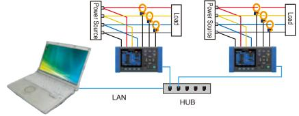
Files recorded in the Clamp On Power Logger's internal memory or SD card are accessible via a LAN or USB connection, and are downloadable using the free **PW3360 Setup and Download Software**.
