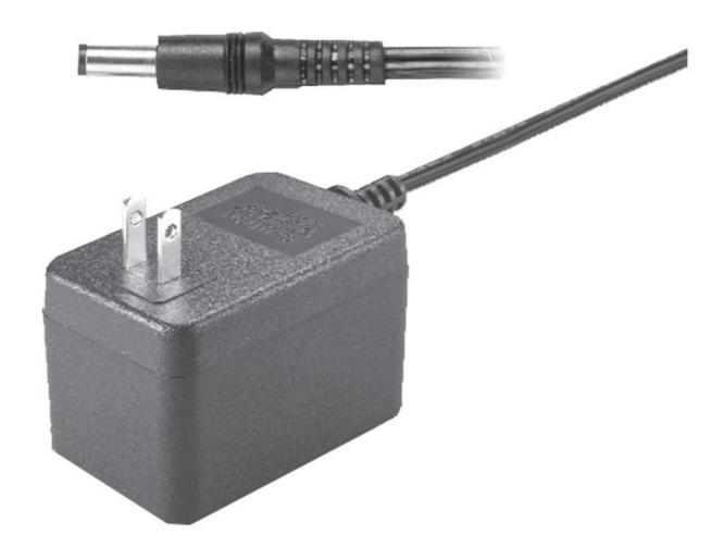
This is an replacement accessory for EC1000 & EC 2000. 25 Watt switching adapter. Output Voltage: 15 VDC. Maximum Load: 1.67 A. Universal input range (90-264 VAC). Frequency: 47 to 63 Hz. Input Current: 0.7 A Maximum. Continuous (Auto Recovery) short circuit protection. Operating Temperature: 0 to 40 °C. Storage Temperature: -20 to 85 °C. Cooling: Natural Convection. Dimensions: 80.5 x 49.06 x 56.00 mm (3.169 x 1.932 x 2.205 Inches). Weight: 280 g (0.62 Pounds).
