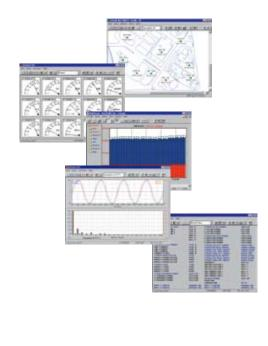
DEDALO software enables power meters to be connected to a PC. It allows to download, to display, to collect and analyse all electrical parameters.
